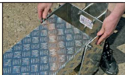
...the right distance. Then use the pin and R-clips to connect the ramps to the towers.
