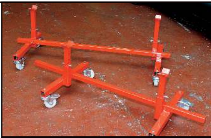
These stands are fully mobile, and both the supports' height and distance apart are adjustable.
