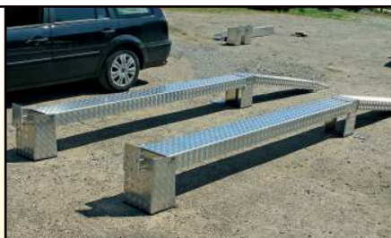
Set the two ramps/platforms a suitable distance apart to match your car's track.
