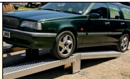
Then simply drive up, apply the handbrake, and – if necessary – remove the two sloping sections.
