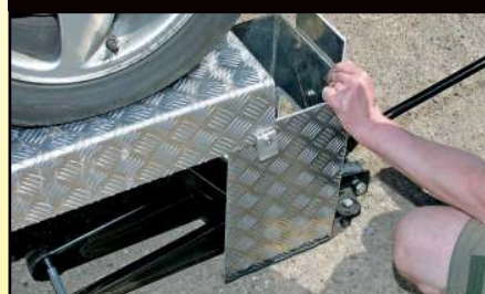
Use a jack under each rear ramp to evenly lift the ramps higher than the front and...
