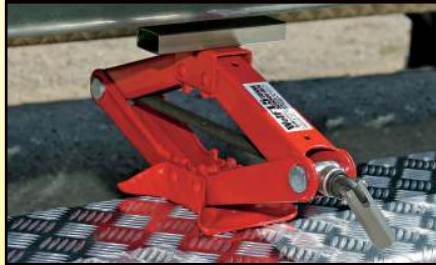
Jacks and stands can be also used to gain access to the sill area or remove wheels.
