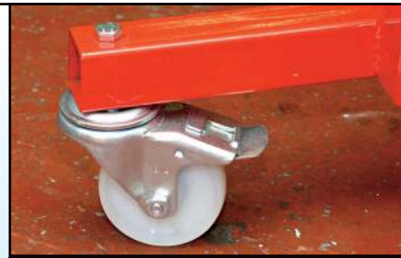
Thanks to the castors, even axle-less projects can be kept mobile. Brakes are fitted too though.
